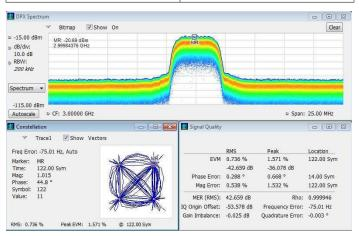
Multi-domain views provide a new level of insight into design or operational problems not possible with conventional analysis solutions. Here vector modulation quality and constellation (Opt. 21) are combined with the continuous monitoring of the DPX® spectrum display.
