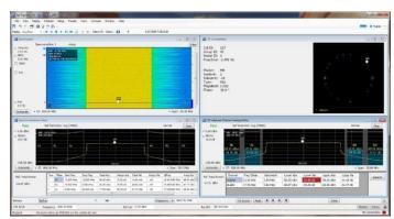
Fast validation of LTE base station transmitter with push button preset, and pass/fail
