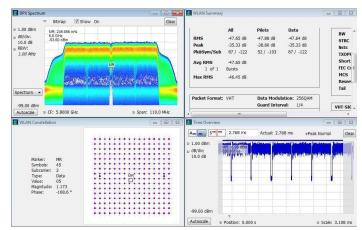
Analysis options for 802.11 standards are available. Here, an 802.11ac 80 MHz signal is analyzed, with displays of constellation, amplitude vs. time, summary of WLAN measurements, and the DPX spectrum of the analyzed signal. The density of the 'shoulders' of the WLAN signal are clearly seen in the DPX display, and a marker was placed on the suppressed center carrier of the signal. An EVM of -47.65 dB and other signal measurements are seen in the summary panel.
